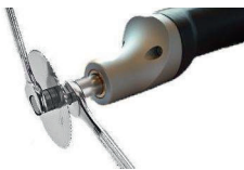
Fig. 1: Releasing the retaining screw
